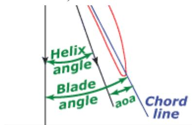
its length. So, normally the standard blade angle is measured at the blade station, 75% of the distance from the hub centre to the blade tip. The angle between the aerofoil chord line and the helical flight path (the relative airflow) at the blade station is the angle of attack and the angle
