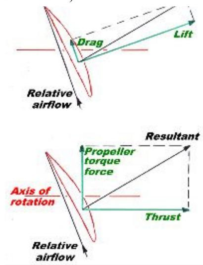
aerodynamic force, in a similar manner to a wing. Consequently, the blades are subject to the same aerodynamics — induced drag, parasite drag, wingtip vortices, lift/drag ratios at varying aoa, pressure distribution changing with aoa, etc. There is a difference in application because, in flight, the propeller has rotational velocity added to the forward velocity. Thus, the flight path of any blade section is a spiral — a helical flight path.
