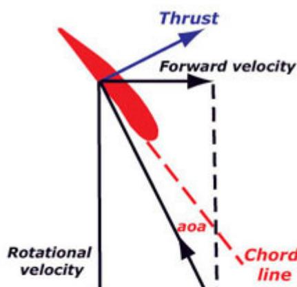
The angle of attack of a fixed-pitch propeller, and thus its thrust, depends on the forward speed of the aircraft and the rotational velocity. Following a non-catastrophic engine failure, the pilot tends to lower the nose so that forward airspeed is maintained while at the same time the rotational velocity of the engine/propeller is winding down. As the forward velocity remains more or less
