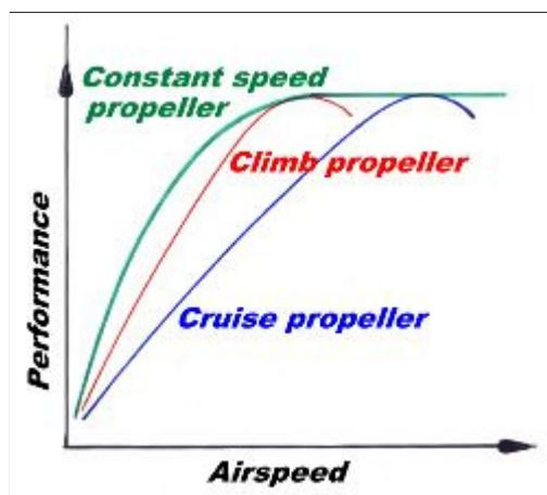
The climb propeller is usually chosen when the aircraft normally operates from a restricted airfield or in high density altitude conditions. The climb propeller will produce maximum efficiency at full throttle around the best rate of climb airspeed and will perform fairly well at take-off. But during the initial take-off acceleration, even the climb propeller may restrict the engine rpm to less than 75% power. The cruise propeller
