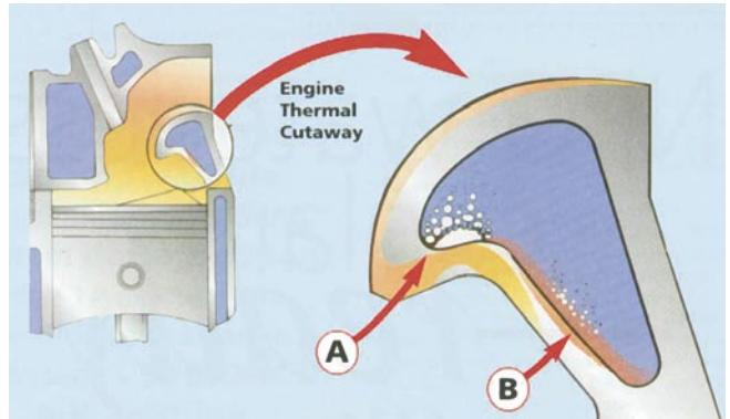
The 9-series heads are made of a heat-treated aluminum alloy. If the head is overheated, the aluminum will soften and warp. Experience has shown that when operating with a conventional coolant/water mix, at CHTs approaching the maximum limit, portions of the head may become hot enough to damage the head after many hours of prolonged high temperature exposure.
