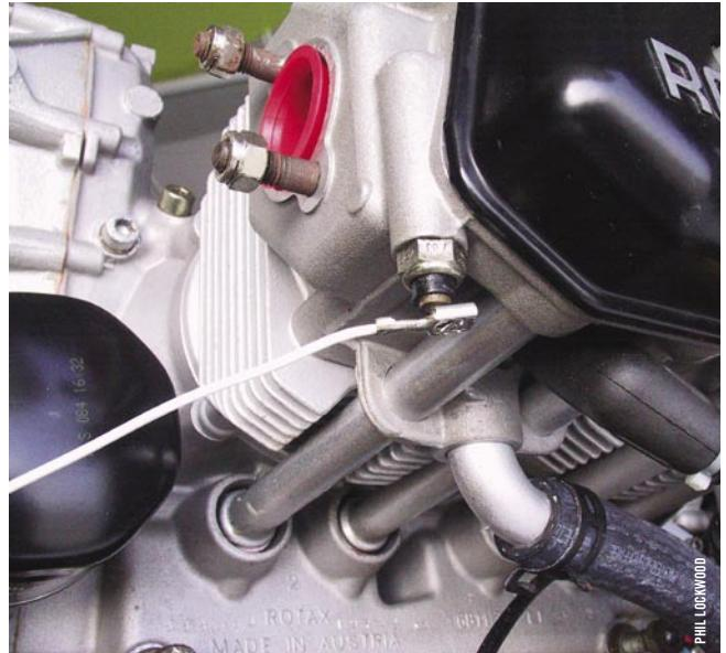
If your CHT never approaches the new 239°F temperature limit, then you could continue to operate with the coolant you have been using. DEX-COOL has been the conventional coolant of choice in North America.
