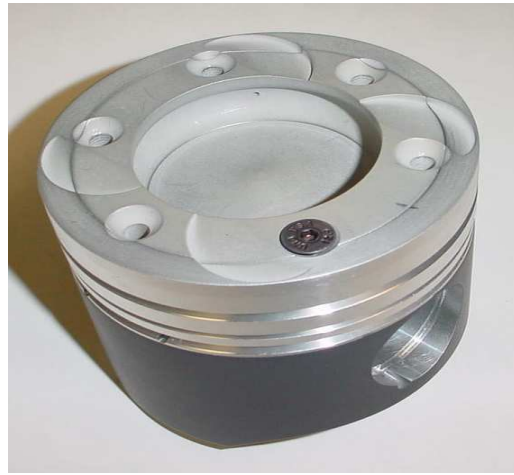
Figure 9 250 Hp SCAI HFE Improved Piston
