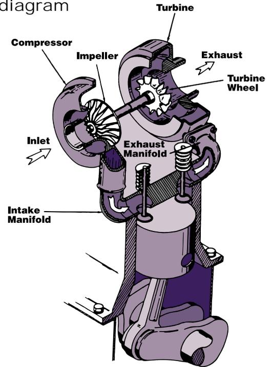
oil leakage is evident, remove the ducting to the compressor inlet and again examine the compressor wheel for blade damage or rubbing on the housing. Also check the radial play and if found to be excessive, remove the turbocharger for overhaul.
