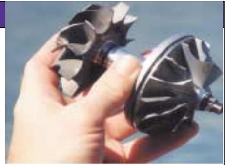
*The driving force of the Kelly Aerospace turbocharger is the turbine wheel (left) and compressor impeller (right). It is capable of rotating up to 120,000 rpm.*
